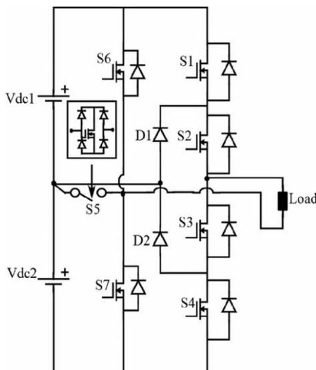
Fig. 2. Proposed fault-tolerant single-phase five-level inverter.
