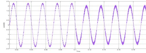
Fig. 7. Output voltage and current waveforms with a transformer due to Vdc2 source failure (Y -axis 200 V/div, 2 A/div; X-axis 20 ms/div).
