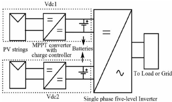
Fig 1. Block diagram of the single-phase five-level inverter.
